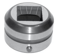
Mate Slug Free Light<sup>™</sup> notches are cut at an angle to create a series of protrusions on the slug. As the slug moves through the die, the protrusions become trapped against the die land to prevent the slug pulling back on to the sheet. (Image enhanced for additional clarity)
