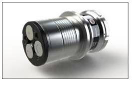
The fully **indexable Ultra IMT<sup>™</sup> 3-Station multi tool** works with Ultra TEC<sup>®</sup> & Ultra<sup>®</sup> QCT<sup>™</sup> B Station punch, strippers and Thick Turret Slug Free<sup>®</sup> dies up to a maximum punch diagonal of 1.250" (31,75 mm). The multi tool can achieve any angle setting on the work piece.
