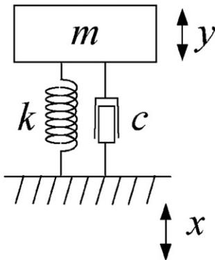
Fig. 2. Dynamic model of a base-excited SDOF system.
