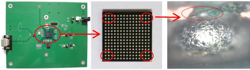
Fig. 5. Micrograph of a failed BGA solder ball with a fatigue crack.
