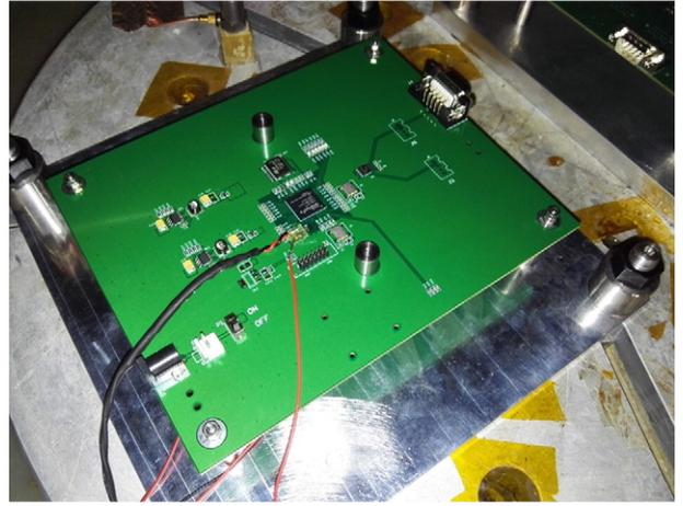
Fig. 3. Specimen of an electronic assembly mounted on a shaker.
