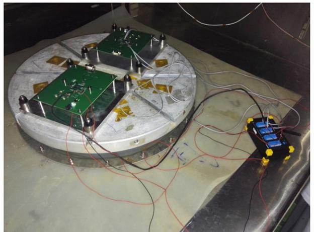
Fig. 4. Experimental setup for a vibration fatigue test.
